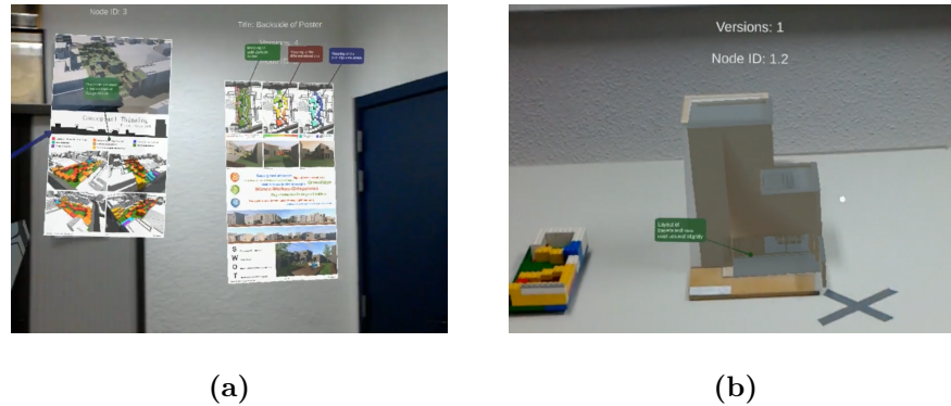
Figure 39: Annotations support for artifacts with (a) multiple annotations giving context on digital artifact parts and (b) an annotation providing context for a real artifact.
