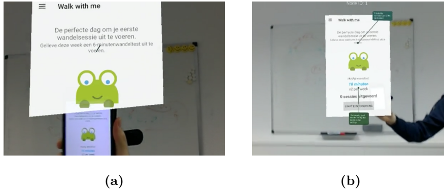
Figure 41: Application view detected by the system using Vuforia with (a) the clipping plane not showing the full screen close-by and (b) the detected screen fully shown in front of the smartphone.
